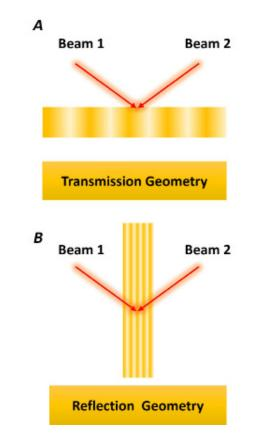
Figure 2. Formation of A) a transmission hologram and B) a reflection hologram.
