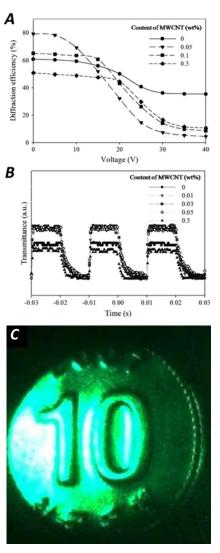
**Figure 6.** Electro-optical properties of the H-PDLC obtained by Kim et al. using a polyurethane-based matrix doped with various MWCNT contents at 40 wt% LC: **A)** driving voltage and **B)** response time at 50 Hz, 30 V. **C)** Photograph showing a reconstructed virtual image of a coin recorded using a H-PDLC obtained at 40 wt% LC with 0.05 wt% MWCNTs. Reprinted (adapted) with permission from *Polym. Int.* **2010**, 59 (9), 1289–1295. Copyright © 2010, John Wiley and Sons.
