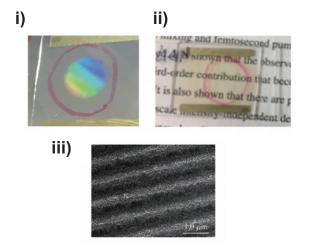
**Figure 5.** Hologram fabricated with photopolymers doped with nanodiamonds by Tomita et al. i) Photograph of the hologram under illumination with white-light, ii) Photogram of the same hologram viewed from the top and iii) from a fluorescent lamp and iii) TEM image of the cross section of the grating. Reprinted (adapted) with permission from *Phys. Rev. Appl.* **2020**, *14* (4), 1. Copyright © 2020, American Physical Society.
