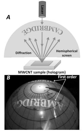
**Figure 7.** Experimental setup and measured diffraction pattern results of the holograms fabricated by Butt and colleagues. **A**) The schematic diagram of the experimental setup employed to capture the diffraction pattern. **B**) The pattern was obtained on a semitransparent hemispherical screen of radius 15 cm by shining a green (532 nm) laser perpendicular to the plane of the CNT array. A clear CAMBRIDGE image was observed in the first order of the diffraction pattern.
