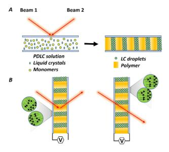
**Figure 4. A)** Formation of gratings in a solution of PDLC: Photopolymerization takes place in bright zones while LCs migrate to dark zones as droplets. **B)** Detailed scheme of the reorientation of the LC droplets in gratings in the presence of an external electric field. When the voltage is off the light is diffracted, while it is transmitted when the voltage is on.
