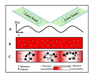
**Figure 3.** Formation of gratings in a photopolymer material: **A**) the sinusoidal illuminating intensity distribution at the plate; **B**) the uniform photopolymer before recording; and **C**) the photopolymer during recording (mass transport and polymer chains). Reprinted with permission from *Polymers* **2017**, *9*(8), 337. Copyright © 2017, MDPI.
