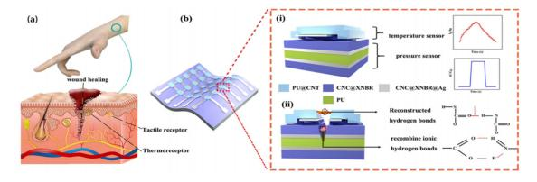
**Figure 2**. (a) Scheme of the human tactile receptors and temperature receptors with self-healing properties. (b) Scheme of the developed self-healable bifunctional e-skin. Adapted with permission from [28]. Copyright 2020 American Chemical Society.
